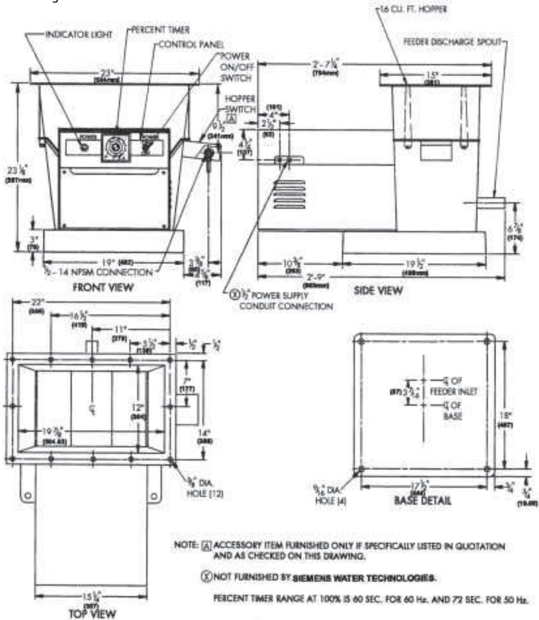
Series 32-050 Percent Timer Controlled Volumetric Feeder
