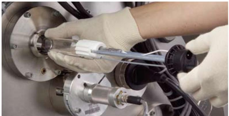
*With hundreds of installations, the TrojanUVSwift™ has demonstrated proven reliability in the field. The system was designed for easy service, and all routine maintenance procedures require access to only one side of the reactor.*
