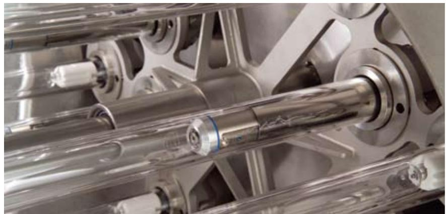
The TrojanUVSwift™ is designed to accommodate one sensor per lamp to allow highly accurate monitoring of UV output and system performance. Systems include a NIST-traceable reference sensor for simple, on-line sensor calibration checks.
