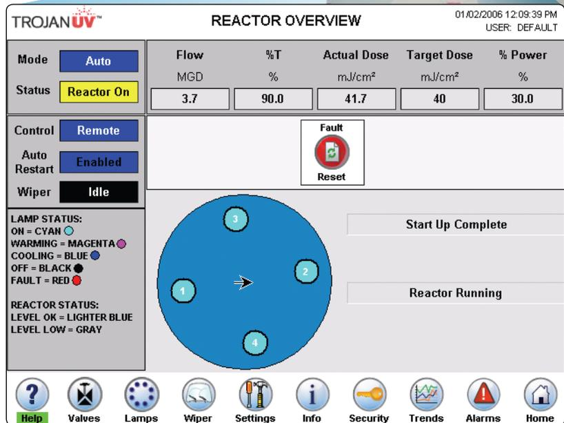
The TrojanUVSwift™ controller is equipped with a robust PLC and touch-screen display configured for user-friendly operation. The system provides dose pacing for optimized disinfection performance and communicates with plant SCADA systems for centralized monitoring.
