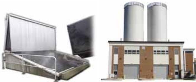
Sliding frame systems, whether used as truck receiving, truck loading, or as intermediate storage, offer a flexible means of storing dewatered biosolids while eliminating bridging and simplifying maintenance. Available in any capacity, with any number of outlets and material discharge rates, sliding frame technology represents the ultimate in design flexibility.
