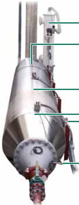
Ammonia scrubber and collection line, 3 gpm of water flow.
