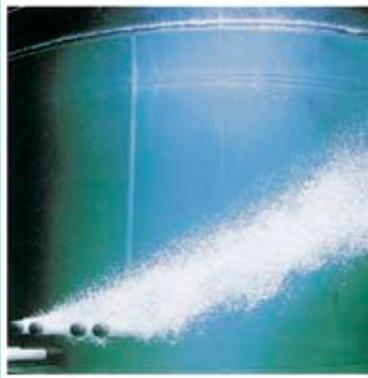
The CSR utilizes rotating diffusers that distribute small air bubbles in a uniform pattern, leading to well dispersed free-rising bubbles that maximize contact time and yield high oxygen transfer.
