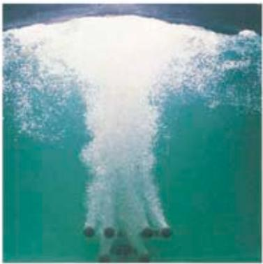
Stationary diffusers alone create a vertical updraft of water, increasing bubble rise rate, reducing contact time, and leading to a coalescence of bubbles that reduces available O<sub>2</sub> surface area for low oxygen transfer.
