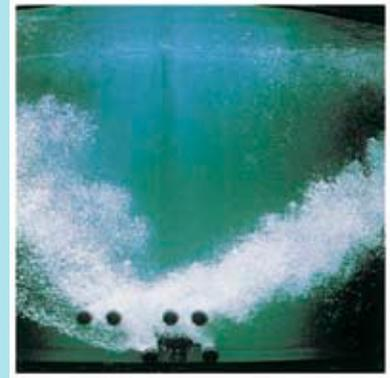
By moving the water horizontally over stationary diffusers, the CSR’s rotating diffusers eliminate the updraft problem created by stationary diffusers alone. The combination of rotating and stationary diffusers can greatly increase aeration capacity for higher basin loadings.
