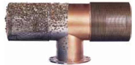
These intake screens can be constructed from various stainless steel alloys and Z-Alloy for both fresh and seawater applications. Different materials can be selected for corrosion issues, to repel mollusks and to resist biofouling.
