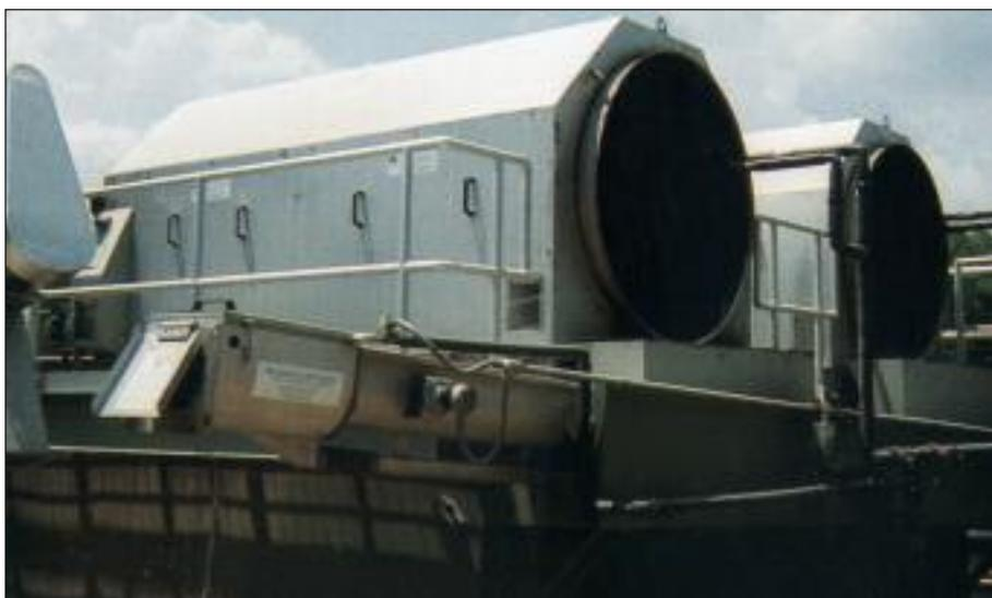
The Hycor® Rotoshear® screen is a high capacity fine screen that was developed over two decades ago. It has been continually updated with new design enhancements; and today, is represented by a complete family of screens. There are ten models with many application
