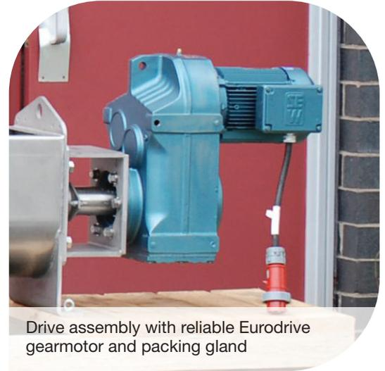
Drive assembly with reliable Eurodrive gearmotor and packing gland
