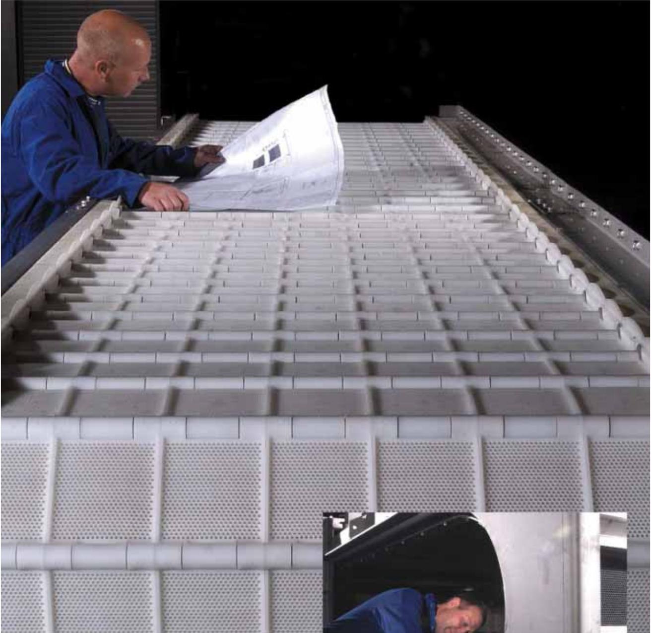
*Fine Screens undergoing final assembly at the Colchester manufacturing facility.*
