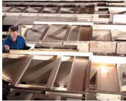
*Band screens under construction at our Colchester facility in the UK.*
