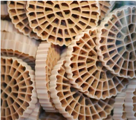
The free-moving plastic carriers in the tank provide an ideal environment for bacteria growth, with aeration providing
