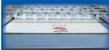
The AQUAbelt® is provided with ARMORDILLO® thickening belts. Application specific weaves and materials are available to optimize liquid/solids separation.
