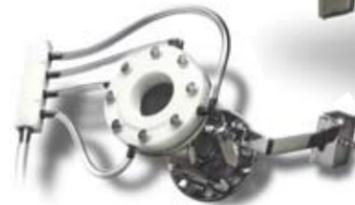
The AQUAbelt® is equipped with a proprietary, variable orifice, in-line polymer mixer. This advanced, non-clog, static mixer is known for its adjustable throat, which provides for application specific mixing energy optimization. Additionally, by virtue of its in-line configuration, mixing energy and retention time, can be optimized independently providing the highest level of performance while using the industry's lowest polymer dosage rates.
