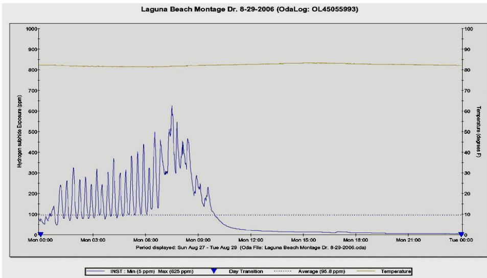
OdaLog showing H<sub>2</sub>S levels before and after start-up of **ECO<sub>2</sub> SuperOxygenation** System
