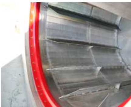
Solids are lifted out by lifting staves
