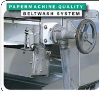
The filter belt wash station on the AQUAbelt® is fitted with a papermachine-quality wash system. Internal cleaning brushes are provided at the cleaning station to keep the shower nozzles open and free flowing. A re-cycle system option is available when enhanced capture rates are needed.
