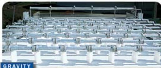
The arrangement of the AQUAbelt® gravity thickening zone ensures the even distribution of the conditioned slurry over the effective width of the moving filter belt.
