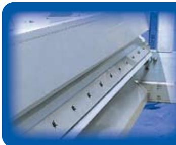
The premium belt scraper employed on the AQUAbelt® effectively removes lumped or partially embedded solids from the belt and serves to extend belt life, while preempting solids carryback.
